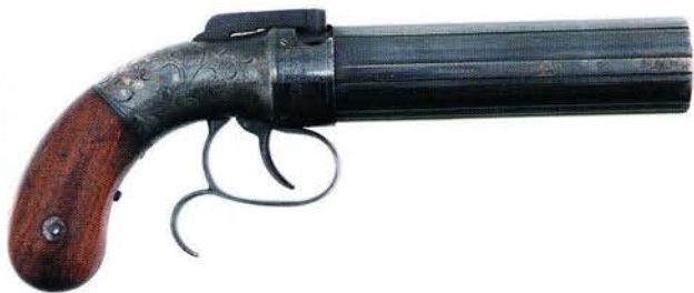
Pepperbox muzzle-loading repeater pistol with percussion lock and multiple barrel. Manufactured by Allen & Thurber, Worcester, Mass., 1847 - 1865. Buffalo Bill Historical Center, Cody, Wyoming. Gift of Olin Corporation, Winchester Arms Collection. 1988.8.2123
