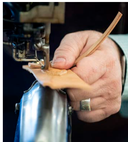
Apprentice Mark Barcus works with a stitcher, a machine built in 1905 and still used for custom leather work.
